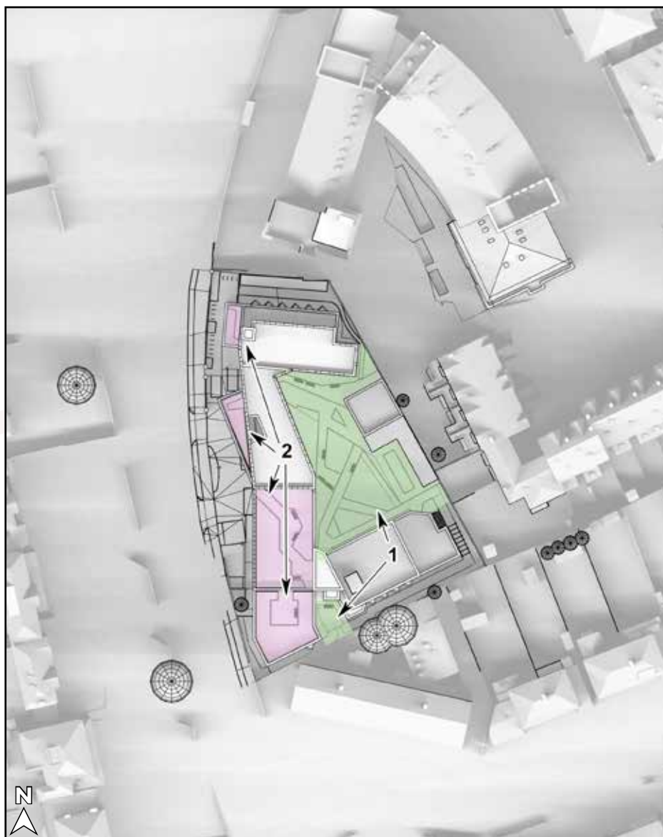
Figure D.7: Indication of the amenity areas that have been analysed (L), Area capable of receiving 2 hours of sunlight on March 21st shown in white (R)
